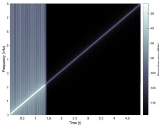
(a) When the chirp signal  $x[n]$  is input, a system gives the output signal  $y[n]$  whose spectrogram is plotted on the left. *12 points*.
